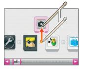
Hold the stylus on the icon you want to move, and slide the stylus up or down to pull the icon out of sequence. You can also press left and right on the ♣Control Pad to select the icon, then press up to move it up.
